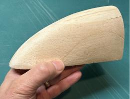
After completing the canopy plug, I mounted it on a length of heavy balsa stick and glued some filler pieces to the stick to take up space in the 2 liter bottle. The photo on the top of the adjoing page roughly shows the next step.
