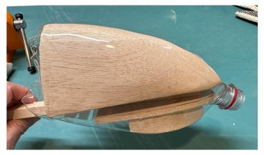
After carefully cutting of the waste portion of the bottle, you will be left with a lightweight canopy that is ready to be glued in place.
