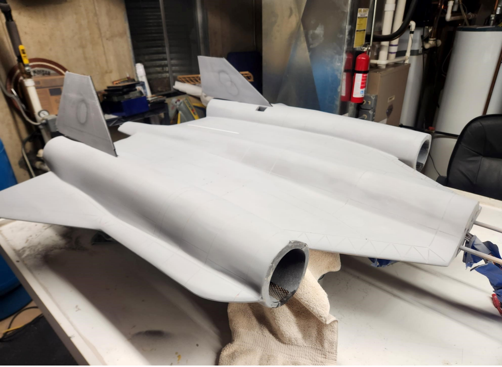
Left: Fiberglass bottom side Right: Hibatu material, brushed the epoxy on top for large surface areas—very smooth after ripping it off. Bottom Left: Primed main body. Bottom Right: All control surface pieces and fuselage. Fans, cones, nozzles, servos, and afterburner lights. My Man Cave
