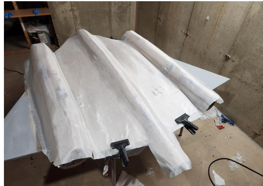
Left: Fiberglass bottom side Right: Hibatu material, brushed the epoxy on top for large surface areas—very smooth after ripping it off. Bottom Left: Primed main body. Bottom Right: All control surface pieces and fuselage. Fans, cones, nozzles, servos, and afterburner lights. My Man Cave
