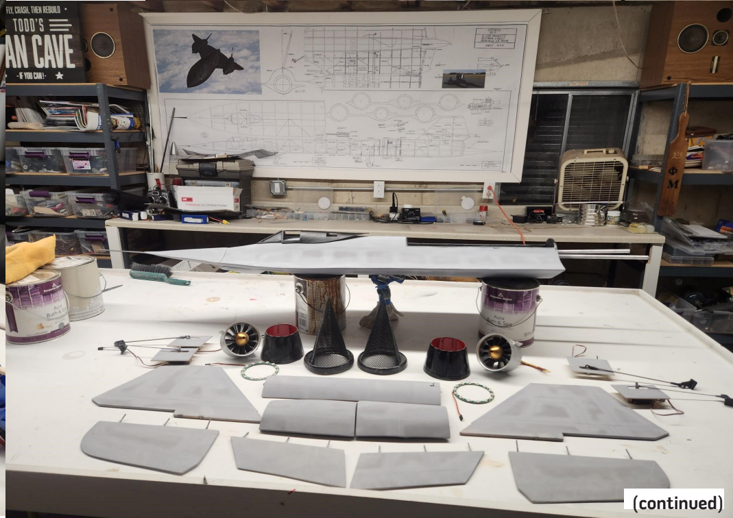
Left: Fiberglass bottom side Right: Hibatu material, brushed the epoxy on top for large surface areas—very smooth after ripping it off. Bottom Left: Primed main body. Bottom Right: All control surface pieces and fuselage. Fans, cones, nozzles, servos, and afterburner lights. My Man Cave
