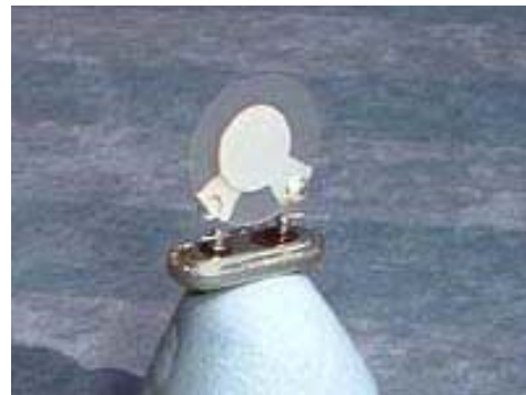
Crystal with metal case removed. The two pins are pushed into blue tack to hold it in place for the photograph.
